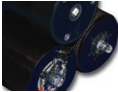
We performed a partial flux measurement technique on three LED package styles (shown in their holders): Philips/Lumileds-Luxeon batwing LED (on top), Osram SMT TopLED (left), and generic T1-3/4 (right).
