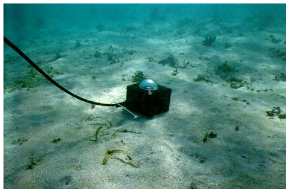
A submerged OL IS-470-WP connected via OL 730-7Q-WP waterproof fiber optic to an OL 756 Portable Spectroradiometer on the surface.
